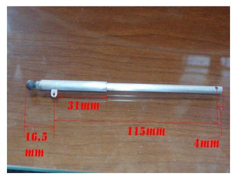
Measure up 115 mm and drill a small hole through the top of the strut. This hole should be at a right angle to the 'D' ring. This will be for the T bar, made from a piece of wire coat hanger.
