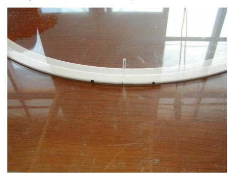
Attach the lower ring to the lower hull. It is best to do this on a glass table top to ensure that the ring stays true and flat. Center the hull half on the ring aligning the mark made earlier with the center of the lower view port. See picture.
