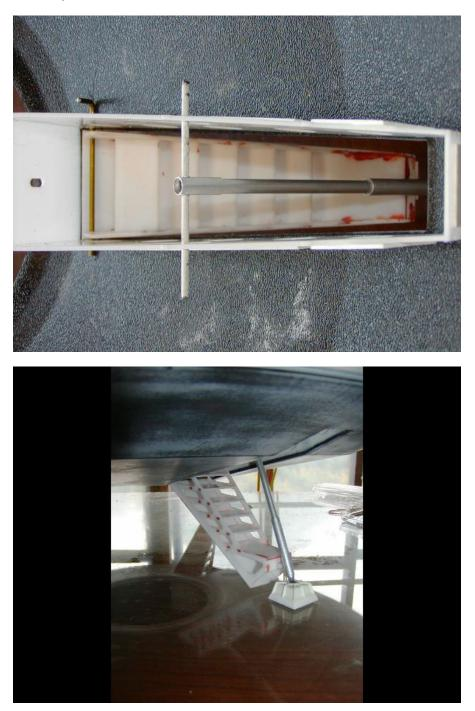
When you're happy with the operation of the gear, install the top of the gear well. It is best to paint the interior of the wells before attaching the top.
