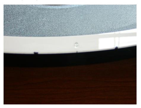
Attach the upper hull half to the upper ring. Align the center the hull with the mark made on the ring half. Make sure to center the hull half on the ring. Align the mark with the center of the main view port. See picture.
