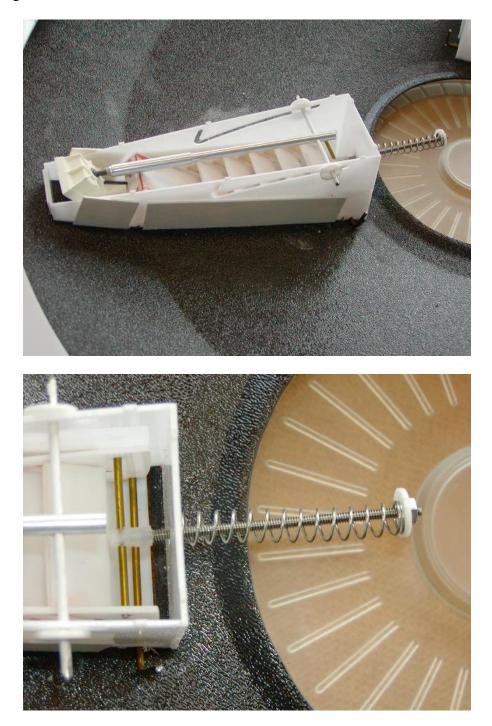
The T bar is fitted to the upper holes in the side walls as shown in picture. The rest is 4-40 all-thread, 70 mm long, and some fittings. The springs were found at a local hardware store. Change this to fit what parts you come up with.
