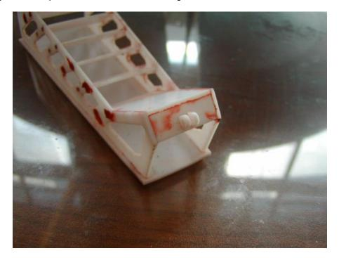
Ensure a good glue joint on these parts as this will be the connecting point between the landing gear and the gear strut.
