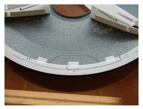
Pictures show the interior in place with a brace made from scraps of sheet plastic for the back end. Do not attach the interior yet.
