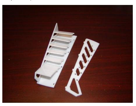
The two small rectangular plates are installed now. One has two slots in it, the other is plain. The side ends will have to be filed slightly to fit between the two side walls. Attach the one with the slots first, setting it flush with the wall edges. The plain one is used as a backing plate. Now attach the two small 'D' rings to the plates. See picture for the assembled configuration.
